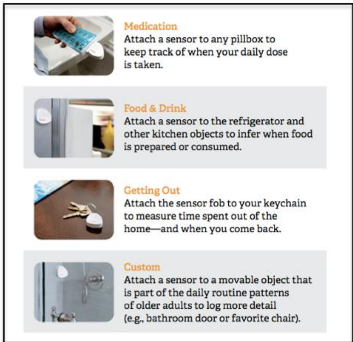
Figure 6. Sensors Placed on Everyday Objects to Monitor Activity 11 (Image source: www.mylively.com )
