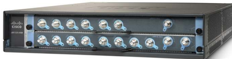
Figure 1. Cisco uBR7225VXR Universal Broadband Router
