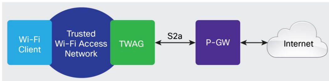
Figure 1. 3GPP Trusted Wi-Fi Integration
