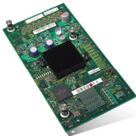
Figure 1. Cisco UCS 82598KR-CI 10 Gigabit Ethernet Adapter
