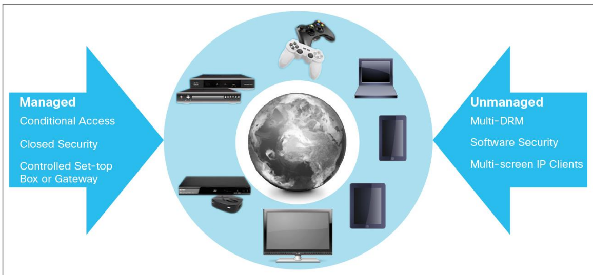
Figure 1. Managed and Unmanaged Networks and Devices
