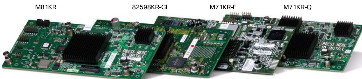
Figure 9. Cisco UCS Network Adapters
