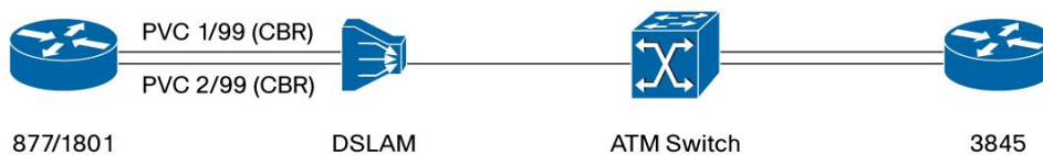
Figure 5. Data Service with Multiple PVCs
