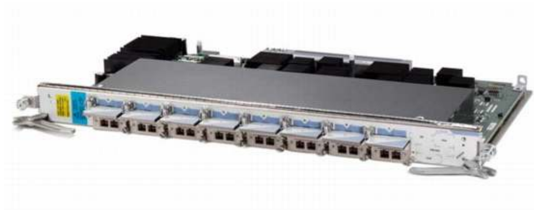
Figure 1. Cisco CRS-1 8-Port 10 Gigabit Ethernet Interface Module
