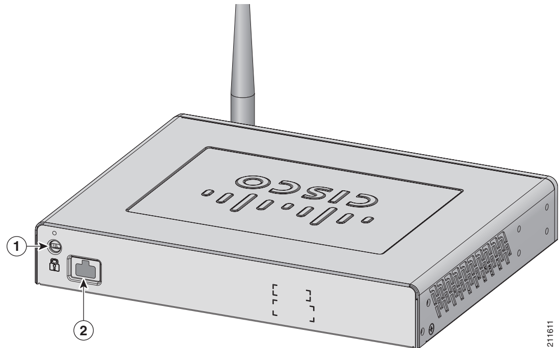
Figure 1-2 Cisco Secure Router 520 Series Router—Back Panel
