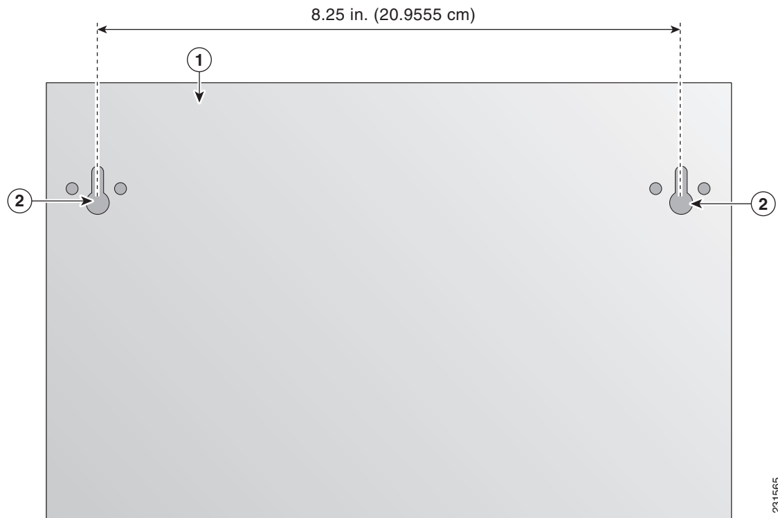
Figure 3-1 Mounting-Screw Holes on the Bottom of the Cisco Secure Router 520 Series Router
