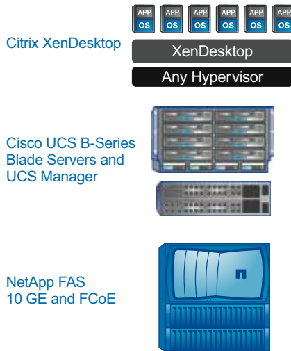
Figure 1. FlexPod DataCenter with Citrix XenDesktop, a prevalidated reference architecture combining NetApp storage, Cisco Unified Computing System (UCS) servers, and Cisco Nexus switches.
