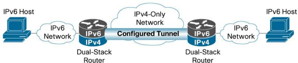
Figure 2. Manually Configured Tunnel Example
