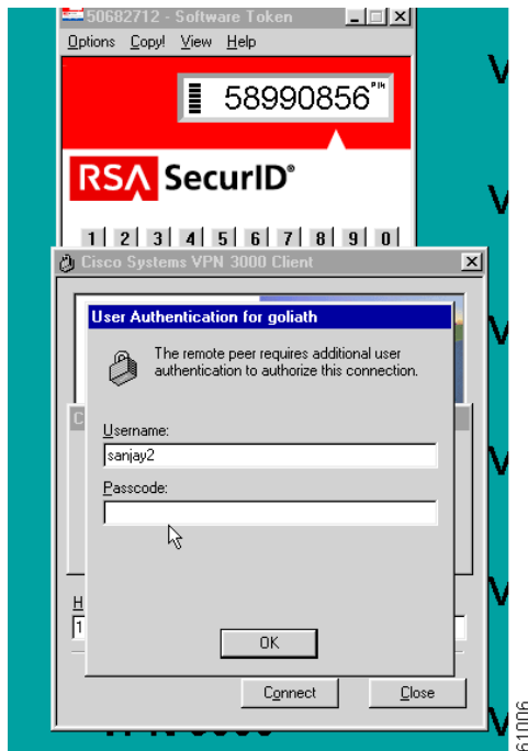
Figure B-2 Software Token Dialog Box—Cisco VPN 3000 Client Version 2.5
