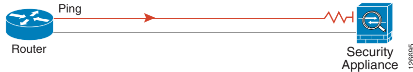
Figure 40-2 Ping Failure at Security Appliance Interface
