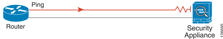
Figure 40-2 Ping Failure at Security Appliance Interface
