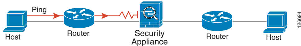
Figure 45-5 Ping Failure Because the Security Appliance is not Translating Addresses
