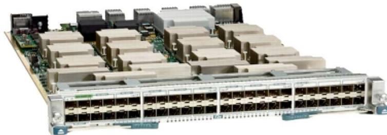
Figure 5. Cisco Nexus 7000 F2e-Series Fiber Module
