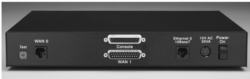
MicroRouter 1250i Back Panel
