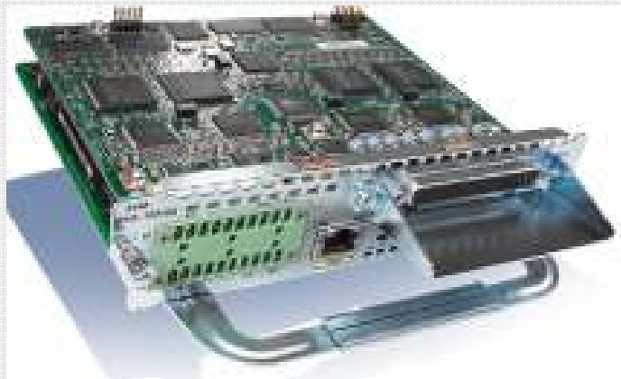
EVM-IPVS-16A: Analog Video Encoding Module
