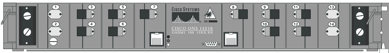
Figure 4 Front-Panel Port Layouts for the Cisco ONS 15216 100-GHz OADM2
