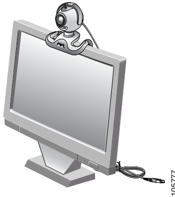
Figure 3-2 Cisco VT Camera Place on PC Monitor
