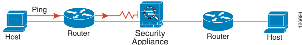
Figure B-5 Ping Failure Because the Security Appliance is not Translating Addresses
