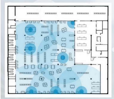
By placing beacons transmitters the receiving unit can be tracked and guided indoor.
