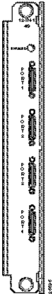
Figure 4-36 12IN1 S4 Back Card Faceplate
