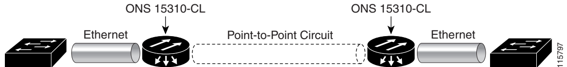
Figure 17-1 CE-100T-8 Point-to-Point Circuit
