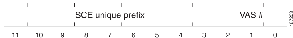
Figure 12-2 VLAN Tag Format
