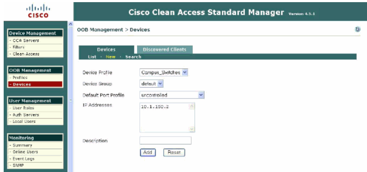
Figure 19: Adding an Edge Switch in the Cisco NAC Manager to Control Using SNMP
