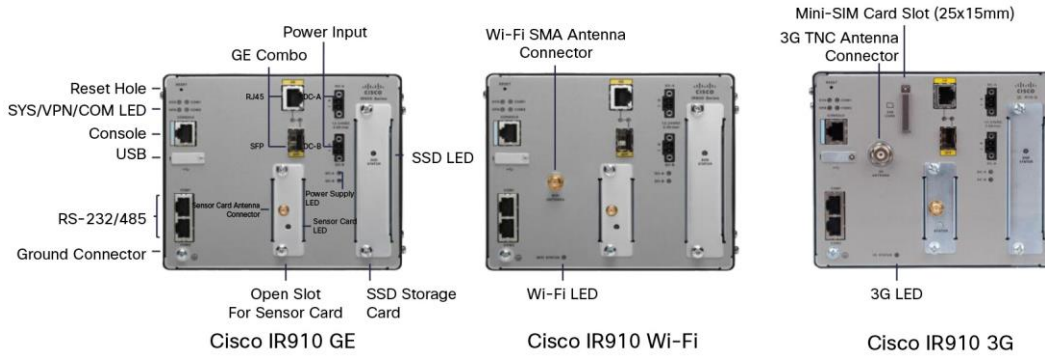
Figure 4. Interfaces and LEDs on Cisco 910 Industrial Router
