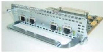
Figure 2. Four-Port Serial Circuit Emulation Network Module (NM-CEM-4SER)
