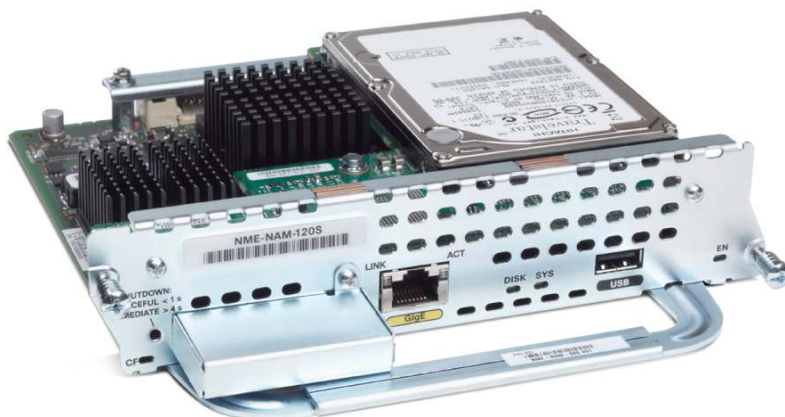
Figure 1. Cisco Branch Routers Series NAM, NME-NAM
