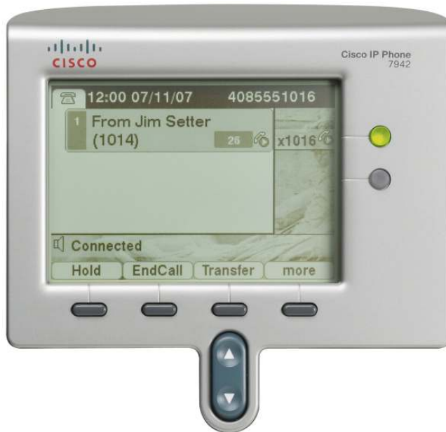
Figure 2. Close-Up of Display and Lighted Line Keys
