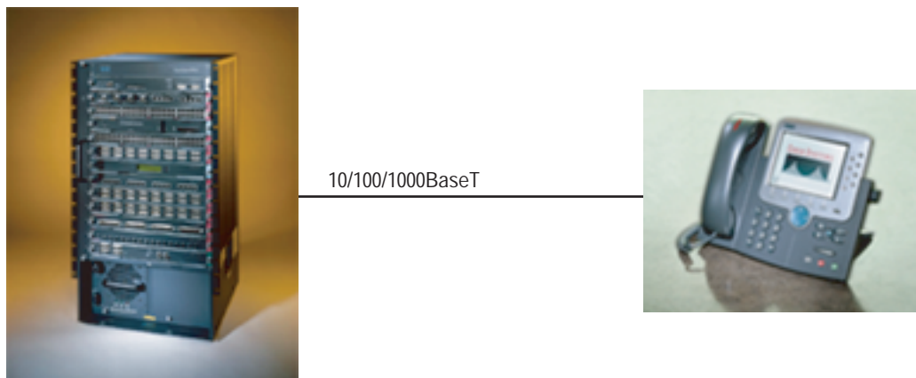
Figure 2 End-Point PSE Power over Ethernet Delivery
