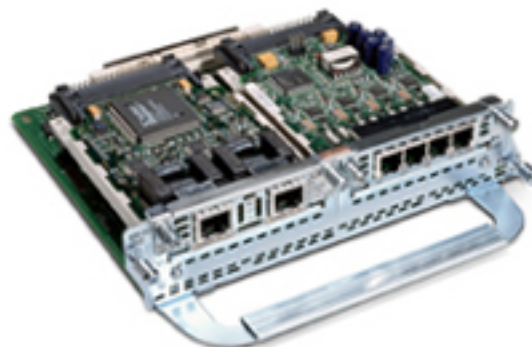
Figure 1 NM-HD-2VE with one VWIC-2MFT and one VIC-4FXS/DID
