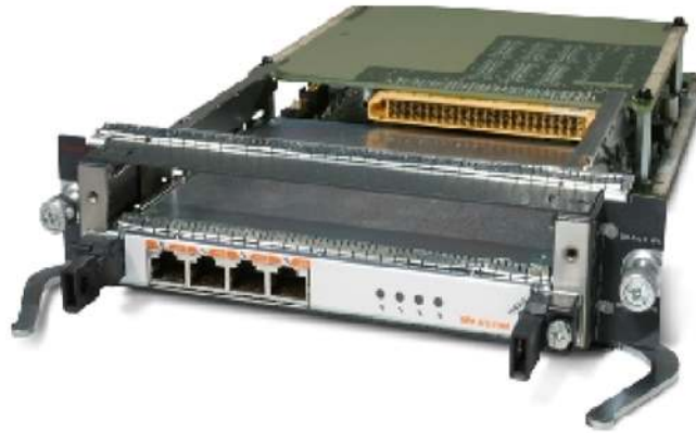
Figure 2. Cisco 7304 SPA MSC with One 10/100 Fast Ethernet SPA
