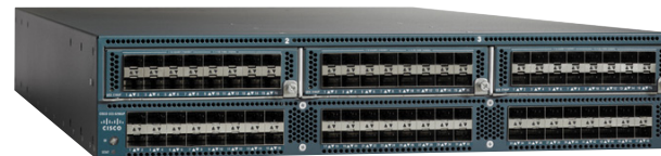
Figure 3. Cisco UCS 6296UP 96-Port Fabric Interconnect
