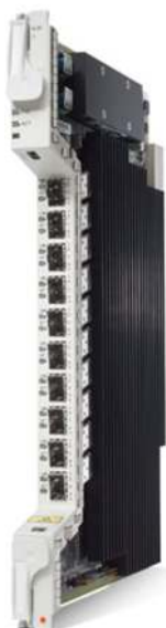
Figure 1. Cisco ML-Series 10-Port Ethernet Multirate Card for Cisco ONS 15454 MSPP
