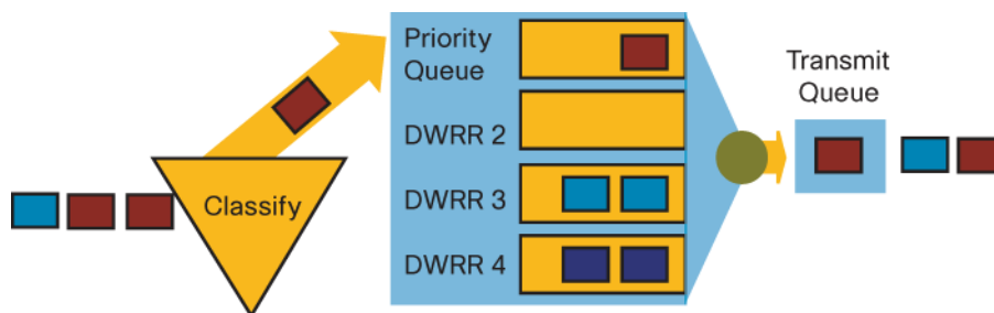
Figure 3. Fibre Channel Port Ingress QoS
