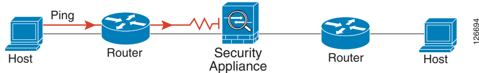
Figure A-5 Ping Failure Because the Security Appliance is not Translating Addresses
