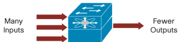
Figure 2. Congestion Caused by Speed Mismatch between Senders & Receivers
