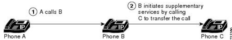
Figure 4: Transfer in a Non-H.450 Environment
