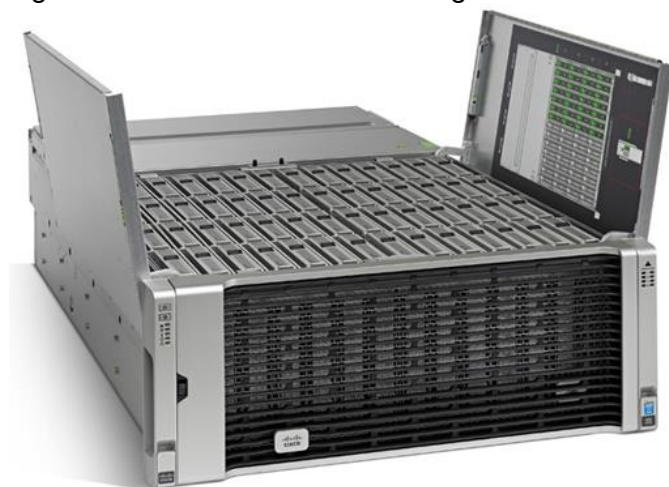
Figure 4 Cisco UCS S3260 Storage Server
