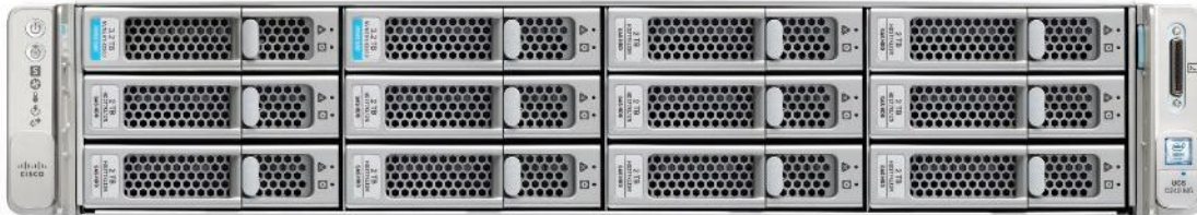
Figure 5 Cisco C240 M5 LFF Server
