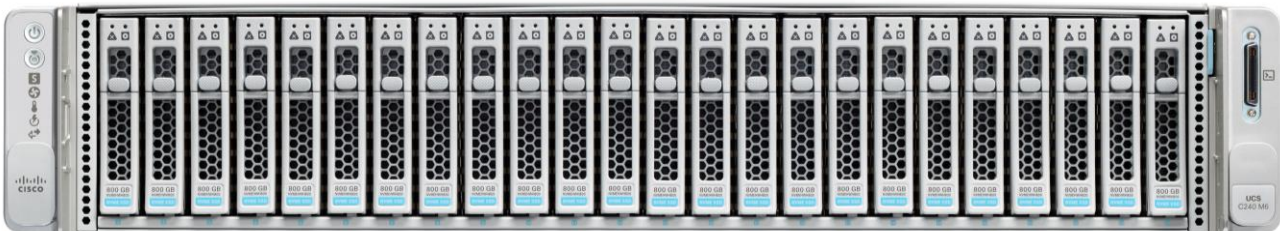
Figure 10. Cisco HyperFlex HXAF240c-M6SN all-NVMe node
