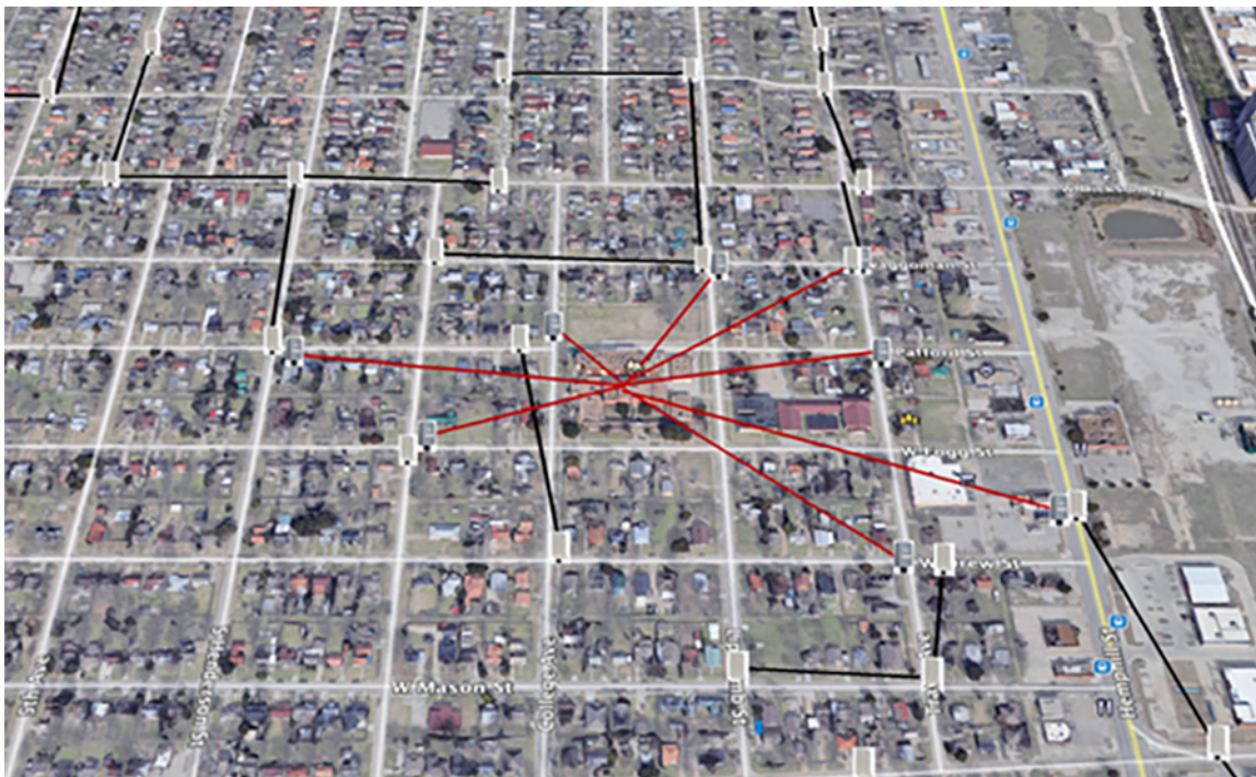
Figure 6 Final mesh radio network path
