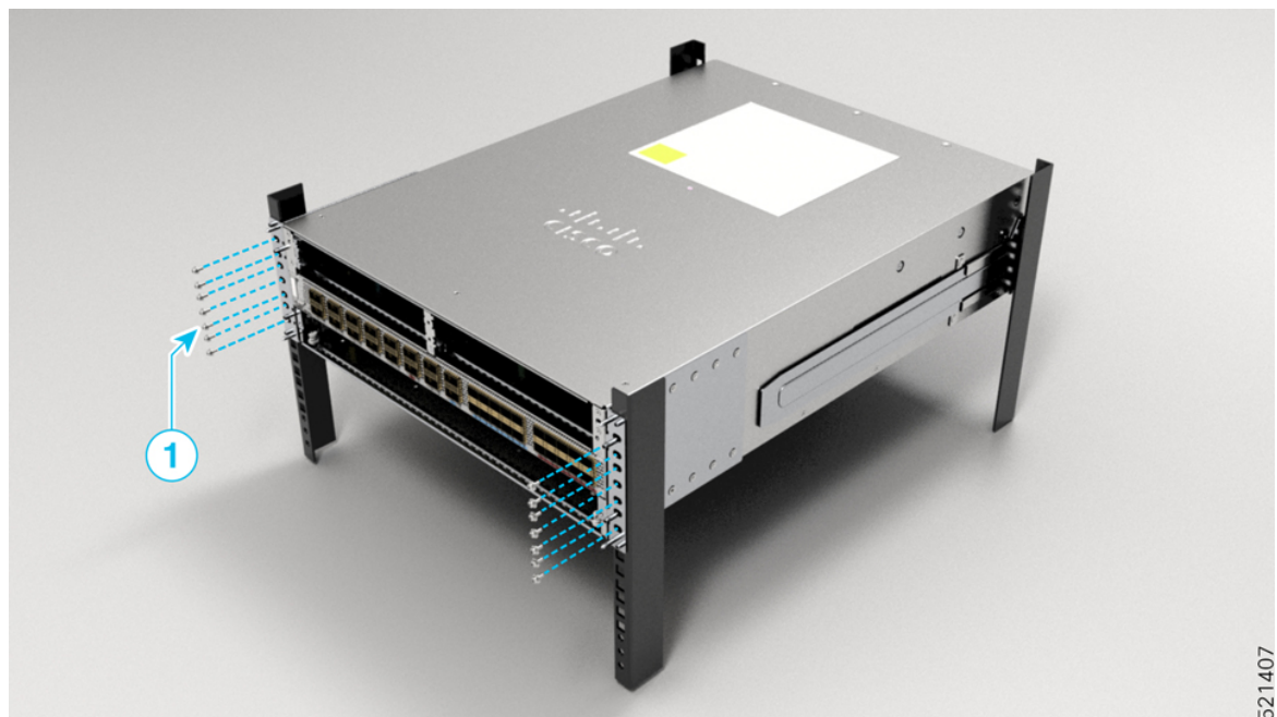
Figure 29: Cisco ASR 9903 Router Mounted in a 4-Post Rack
