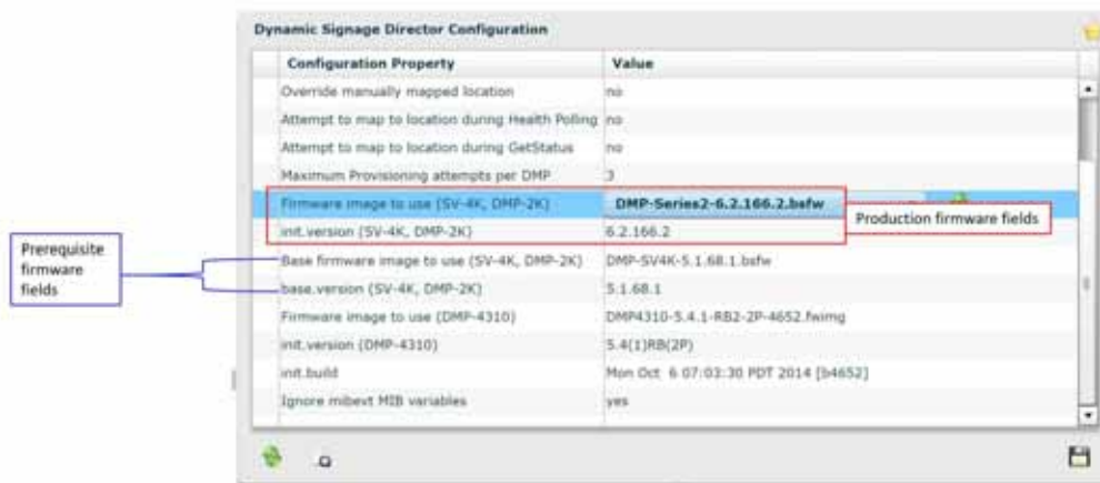
Figure 4 Firmware Image and Version Properties Required to Provision the SV-4K and DMP-2K
