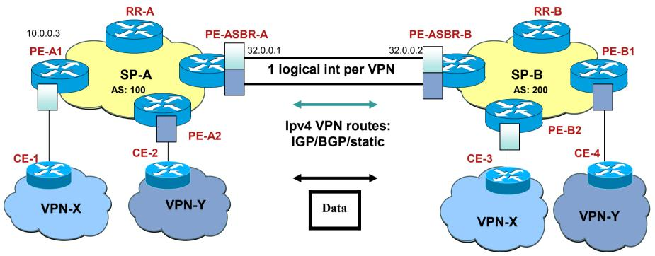
>Simple Concept (extension to Basic VPN – RFC 2547). Each ASBR treats peer ASBR as a CE.
