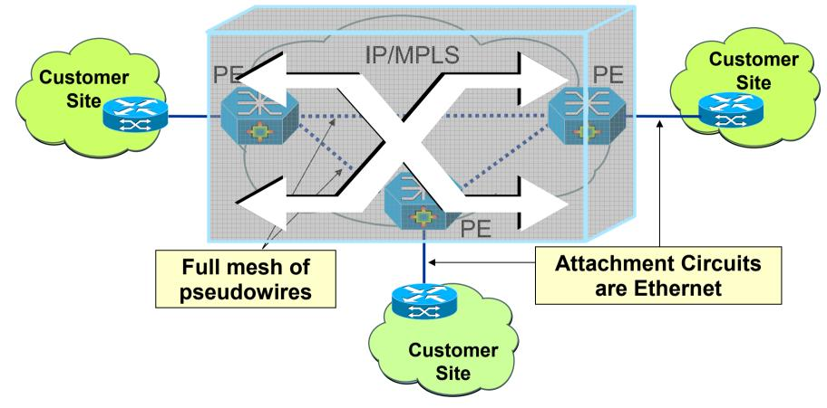
The set of PE devices interconnected via PWs appears as a single emulated LAN to a customer
