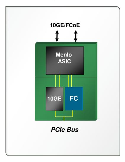
Menlo ASIC – Nexus designed multiplexer and FCoE offload protocol engine
