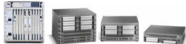
ESR 10000 – Centralized BRAS ASR 1000 – Distributed BRAS
