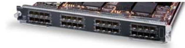
Storage Services Module
