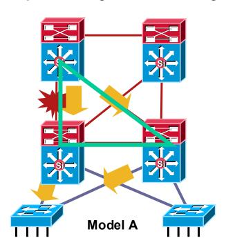
**Squares:** Link/Box Failure Requires Routing Protocol Convergence
