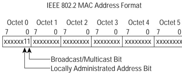
If this bit is set, the MAC frame is destined either for an arbitrary group of hosts or all hosts on the network (if the MAC destination address is the broadcast address 0xFFFF.FFFF.FFFF). IP multicasting at Layer 2 uses this capability to transmit IP multicast packets to a group of hosts on a LAN segment.
